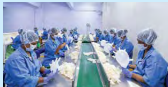
Airtight Test for Detecting Pinholes & Visual Defects
