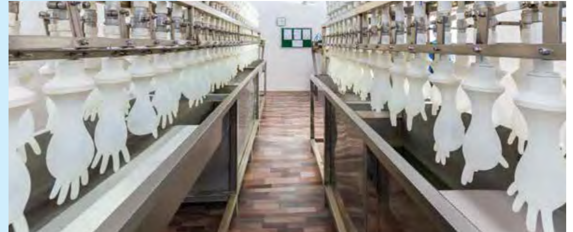
Watertight Test to ensure compliance with Global AQL Standards
